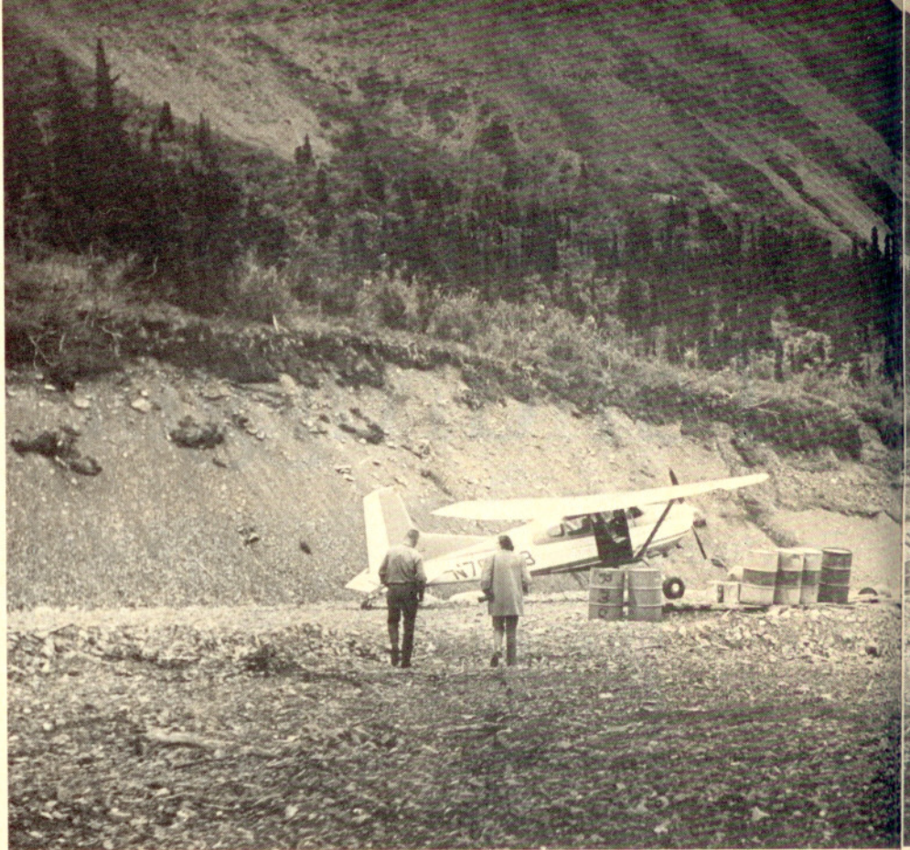
The taildragger's ground-handling eccentricities can be far outweighed by its virtues when it comes to operating into unimproved airstrips. This Cessna 185 has just put down at a river-bottom airport near Northway, Alaska.
